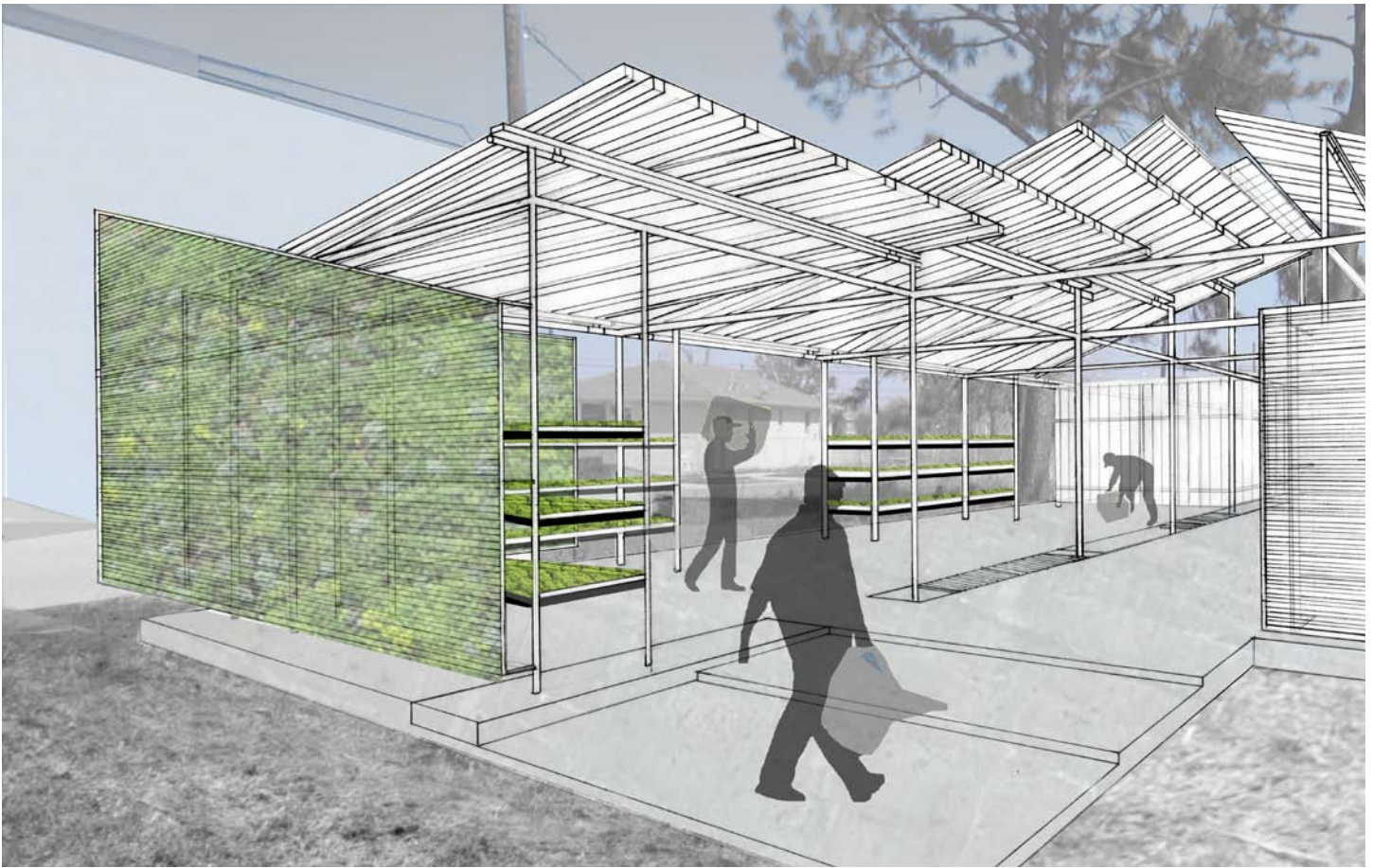
Above: Entrance perspective displaying unconditioned growing beds and oscillating roof structure. Below: View of the operable wall system from the unconditioned growing space.
